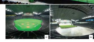
The scene changing from baseball mode (01) to soccer mode is a masterpiece. The natural turf on the baseball field is rolled up, and a huge natural turf stage measuring 120m long, 85m wide, and weighing 8,300t is lifted 7.5cm by air pressure and moves at 4m per minute using 34 wheels. (02)
